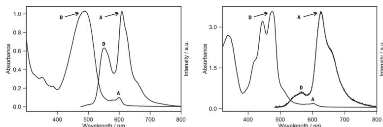
**Figure 2.** Left: Absorption and emission spectrum of a ZeoFRET® sample with a D:A ratio of 33. Right: The same for a sample with a D:A ratio of 52. The emission was measured upon excitation of D at 450 nm.
